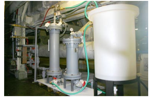
A backwash filter system was designed and constructed for a pilot-scale test.
